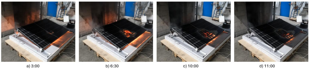
Figure A 6 – MT6 with 1.5 mm PVC membrane, 6 mm cement board and 100 mm EPS insulation. Time from ignition in min:sec.
