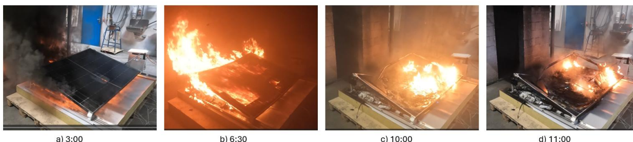
Figure 8 – MT4 with 1.5 mm PVC membrane on top of 100 mm mineral wool insulation. Time from ignition in min:sec.
